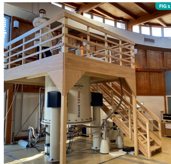
FIG 1. The new 1.2 GHz NMR spectrometer at Instruct-IT.
