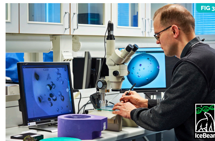
FIG 3. Instruct Centre FI Scientist Dr Kristian Koski fishing out crystals for data collection and tracking the samples simultaneously with the IceBear software at the Instruct ERIC Centre FI, University of Oulu.
